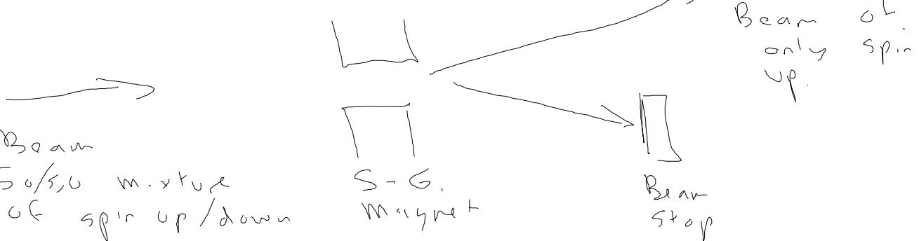
Note S-G magnet has a strong non-uniform field in only one direction. Thus can prepare only one component of spin.
